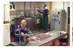
**Specialised Cleaning Processes** Pvrolitic and Ultrasonic cleaning cycles to remove carbon depositation.
