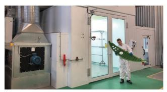
which is controlled by a bespoke PLC system and incorporates electronic data logging to record temperature, humidity and cycle outputs in addition to a standalone temperature control for increased safety.
