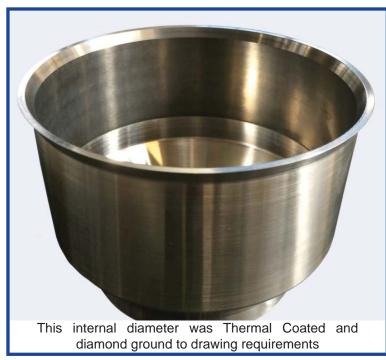
as Hard Chrome Plating. There are many advantages of thermal coating over hard chrome plating such as; reduced health and safety risks, excellent repeatability due to robotic control and lower environmental impact due to a reduction in hazardous waste generation.
