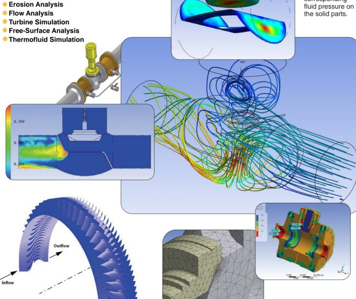
Turbine blade simulation using CFD to determine efficiency, and also to analyse blade stress and deformation.
