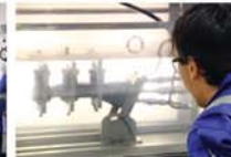
Pressure Testing External envelope and internal circuit integrity testing.
