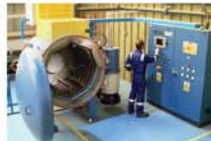
Vacuum Brazing and Heat Treatment Advanced repair schemes and manufacturing techniques.
